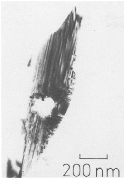
Figure 7 Laves phase precipitate with M_{23}C_6 nucleus.
