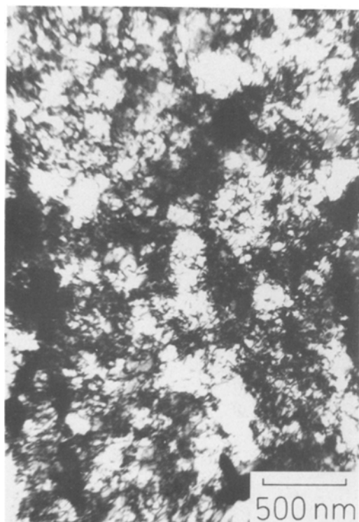
Figure 19 Thin foil from accelerated creep test specimen, showing very high dislocation density.
