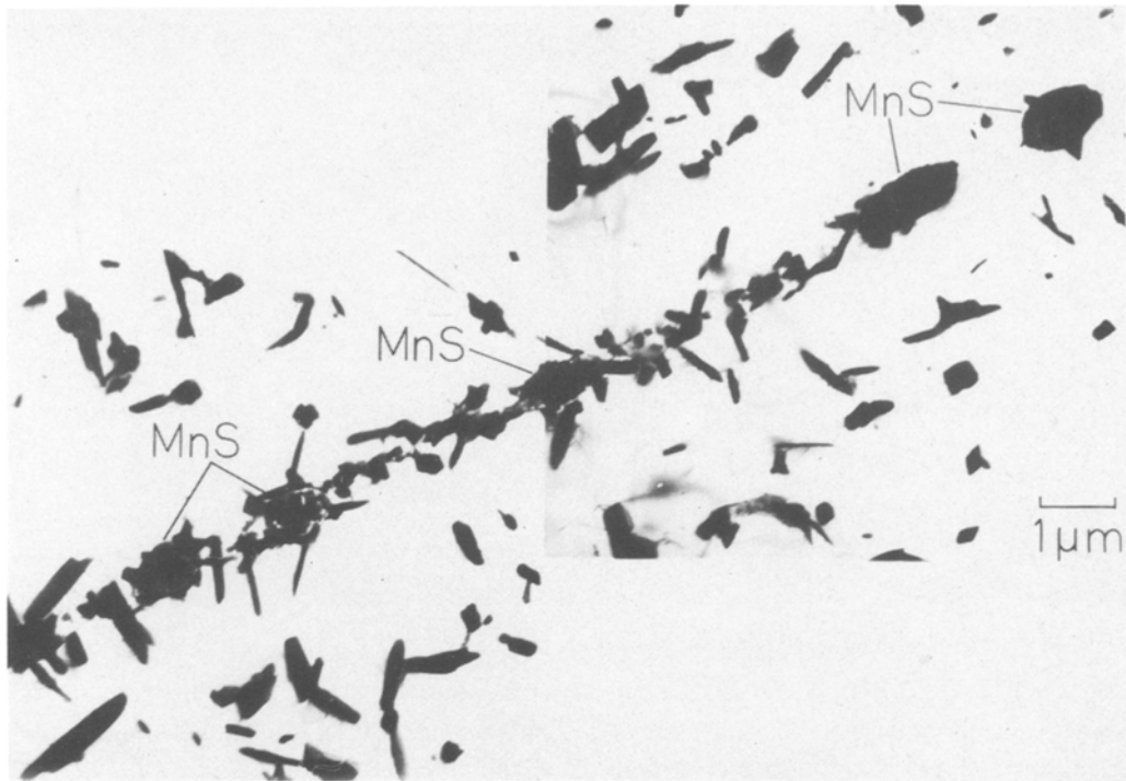
Figure 5 Precipitate denuded zone adjacent to MnS.
